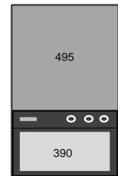
Taller 900mmH Microwave Wall Widths (mm) 600
